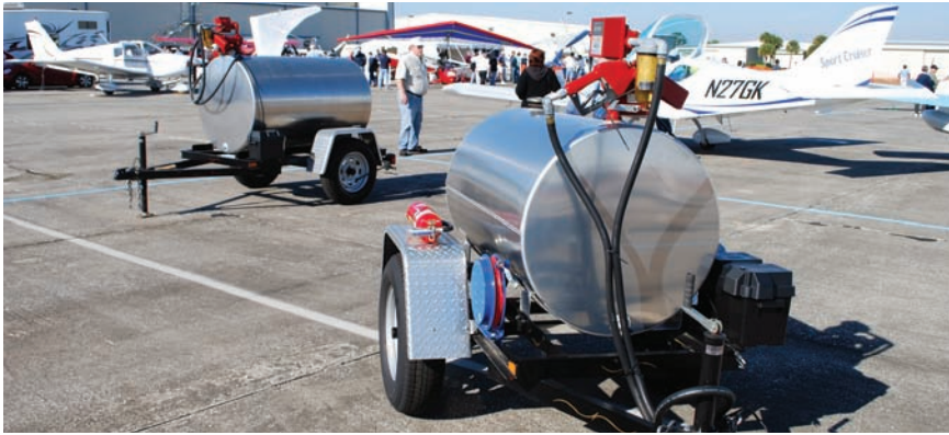
At this year's U.S. Sport Aviation Expo at Sebring, Florida, Jet Fleet Management (Fort Lauderdale, Florida, http://JetFleetMgmt.com ) displayed 150-, 280-, and 500-gallon capacity fuel trailers aimed at those who burn autogas.
