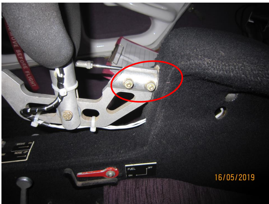
Figure 3 – Location of tube to inspect
