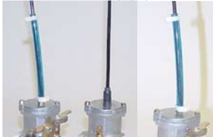
Figure #9 – Special attention needs to be given to the Carb top entry. The use of a short length of ¼" i.d. fuel line makes and excellent strain reliever.
