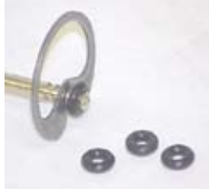
Figure #7 – Pay particular attention to the relationship between the tuning pin and the e-clip. These two parts will rotate and wear from vibration. The small o-ring shown here provides enough interference to stop this wear.
